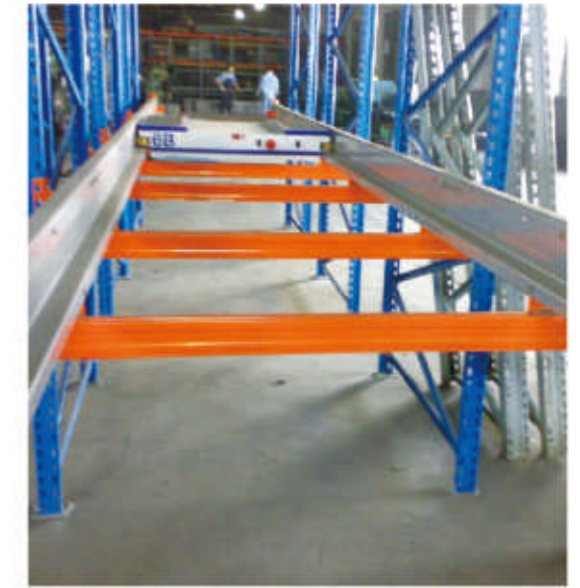
Shuttle car can move the pallet from the depth of the tray to the front, use the forklift to take down the goods.
