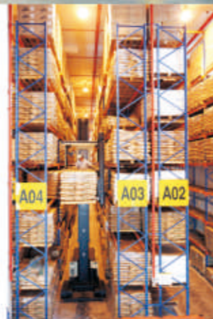
Very Narrow Aisle Rack Configuration
